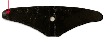
Electrode with Gel Missing
